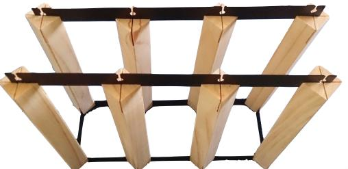
Take Care to ensure that the metal frames continue to align with the pre-cut notches in the wooden rails. This will ensure much easier assembly in the following step.
