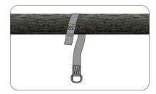
3. Pull the D-ring end through the loop end. Tighten the straps by pulling down firmly.
