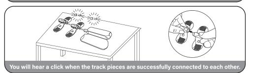
Snap the tracks together at an angle instead of pushing them in straight.
