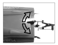
1. Twist the cabin cover switch to left or right, and then forced upward to lift the cabin cover.
