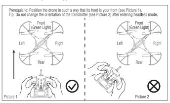
To turn on Headless Mode: Press the Headless Mode button. The LED light of your drone will flash which indicates the drone has entered Headless Mode. To turn off Headless Mode: Press the Headless Mode button again and the drone LED lights will remain a solid light which indicates that the Headless Mode is off.
