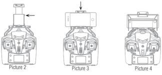
3. Insert the lens hood into the slot and make sure the lower edge of the lens hood is as close to the mobile phone as possible (Picture 4).
