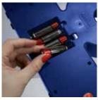
Place 4 (AA) batteries following the battery polarity diagram shown in the compartment.
