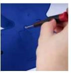
If using batteries to power the device, unscrew the battery cover with a Phillips screwdriver (not included).
