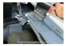
**Step 3:** Open the hood of the truck and locate the bolt on the driver side hood rail where the mount will attach.
