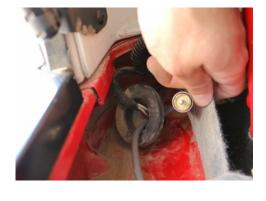
**Step 6:** Place the Teraflex CB mount between the tail light housing and the Jeep. With the coax cable routed out of the round notch on the bottom of the CB mount, reinstall the three mounting screws into the tail light and secure the mount and tail light to the Jeep.
