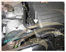
4- Loosen and remove the air box mounting screw. This screw will be reused.
