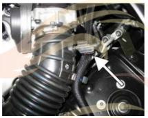
2- Loosen hose clamp at the throttle body.
