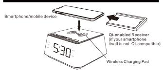
An 5W Wireless Charging Pad is built on top of this unit for wireless power transfer to any Qi-compatible Smartphones or Qi-enabled Receivers over a vertical distance of not more than 0.2 inches (5 mm).
