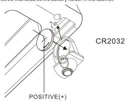
6.) Turn the radio right side up and confirm that the LOW BATT indicator is 'Off'. 7.) Save these instructions. You'll have to do this again five to eight years from Now! WARNING: DANGER OF EXPLOSION IF BATTERY IS INCORRECTLY REPLACED. REPLACE ONLY WITH THE SAME OR EQUIVALENT TYPE
