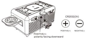
The lithium backup battery needs replacement when the LOW BATTERY indicator flashes, otherwise, the time and alarm settings will be lost/reset after a power outage.
