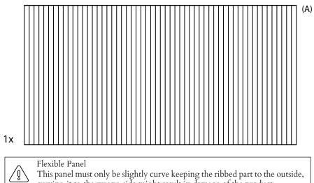
This panel must only be slightly curve keeping the ribbed part to the outside, curving it to the wrong side might result in damage of the product.
