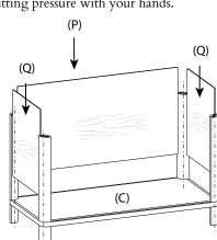
Insert the screws to the base (C).
