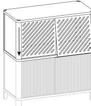
Metal doors (N) are reversible creating four different pattern combinations. You can flip them to have the one you prefer facing the front. Metal doors are rectangular, position the longer side vertically.
