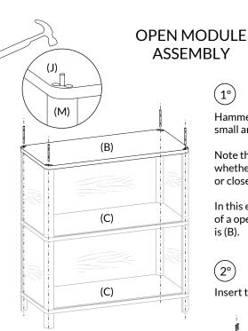
Hammer in the metal cylinders (J) with small and gentle blows.
