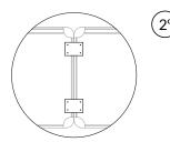
Screw the pieces as close to the legs (K) as possible, making sure one half of the piece is in one base and the other half in the other base.
