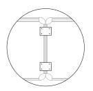
Screw the pieces as close to the legs (K) as possible, making sure one half of the piece is in one base and the other half in the other base.
