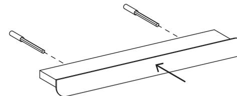
Insert the shelf into the shelf supports that are now fixed to the wall. The shelf is held in place by pressure. If necessary, give small taps to secure its position.
