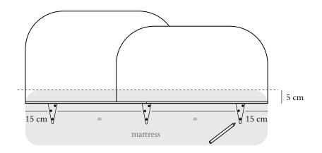
Screw the angle brackets (H) to the wall (x9 wall plugs and x9 screws).
