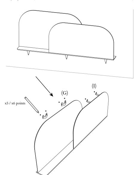
Put the headboard on the floor to make the holes marked in the previous step and screw the fitting to the wall (x5 / x6 wall plugs and x4 screws).
