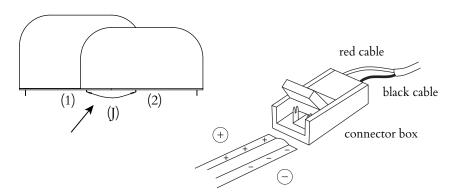
You will have received a pre-assembled connection cable (K+L+M) that allows you to connect the LEDs to the wall socket. Connect the end of the LED strip of your back panel to the beginning of the cable (K) using the connector box. Do this in the same way you did in the previous step.
