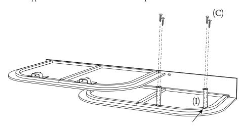
The angle brackets that support the headboard will be located about 5 cm below the mattress. From there, mark the screw holes (9 holes) of the angle brackets with a pencil 15 cm inward from each end, and mark the midpoint to center where the headboard will go.
