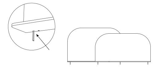
Now we will link the LED strips of the back and front panels together using piece J. On piece J, flip open the top part of one of its connector boxes. Take the end of the front panel's LED strip (1) and place it inside de connector box you just opened.
