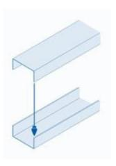
Screw the channel using Wickes Drywall Screws directly to a timber floor or drill, plug and screw using Wickes Nailable Plugs into a level concrete floor. The screws should penetrate the timber by at least 30mm. If a subfloor is particularly uneven it is recommended that a timber "sole plate" the width of the channel (52 or 72mm) and at least 30mm thick should be secured to the floor, and then the track to the timber. Pack the timber out as necessary to achieve a level base.
