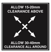
Using a blunt object push the speaker cover to open it up completely. Allow 15-20mm clearance above the cover and 30 - 40mm clearance all around.
