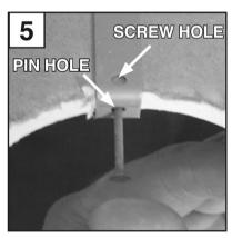
Whilst holding a fitting clip, align the pin hole with 12mm plasterboard and push one of the supplied fixing pins through the hole and into the plasterboard until fastened in place. Use optional No.6 screws in 9mm plasterboard.
