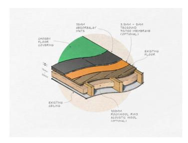
Absorbalay is made of a bespoke closed-cell polymer layer, sandwiched between two sheets of high-mass acoustic barrier. This not only provides both impact and airborne protection, but also provides insulation across a much wider range of frequencies.
