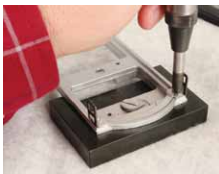
The same tools are used for Alco frames with the same professional results.
