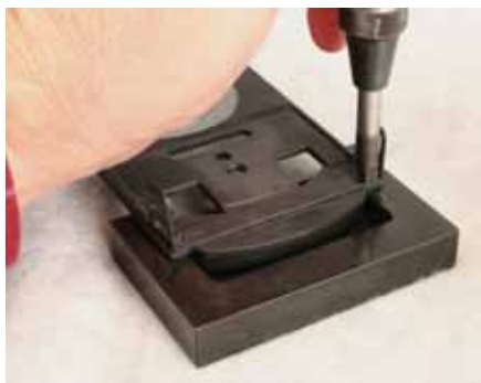
The BR-FB Fitted Base for F3 and Alco frames provides firm support for securing ladders to the frames. Here, an F3 frame is inserted and the ladder stake is being re-swaged using the Super Riveter with the BRT4-2 Swaging Tip.
