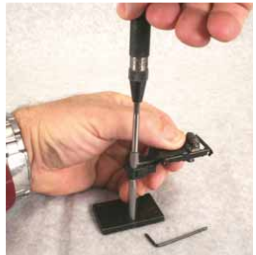
Peening rivet for knuckle pin on knuckle coupler using Original Riveter with BRT1-1 Tip and the BR1-P1 Backing Stake. Parts needed for this fix are Coupler Knuckle Spring #480-16 and Coupler Knuckle Pin #TC-23. Get lots of the tiny springs. They get lost so-o-o easily!
