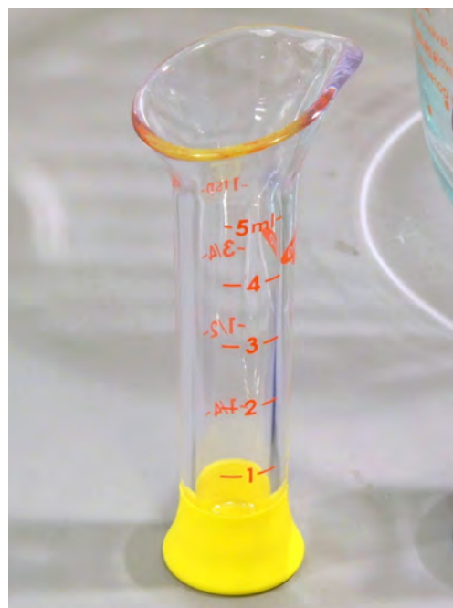
3-8. I find the smallest graduated beaker in the beaker set I got from Amazon to be especially useful for working with the typically smaller quantities of model paint. This beaker goes all the way down to one milliliter (less than a quarter teaspoon). See the text for details on how to find this beaker set online.
