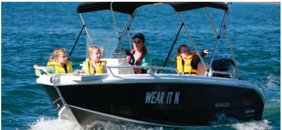
Vessel registration numbers/letters (in this case WEAR IT N) must be displayed on both sides of the hull.
