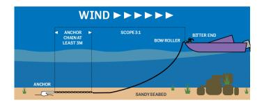
Nylon and silver rope are both suitable materials for anchor lines. Nylon is best for strength and stretching ability and is also more resistant to abrasion. Silver rope has less tensile strength.
