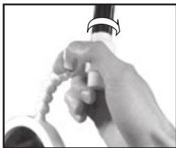
Screw mirror connector clockwise onto shower pipe.
