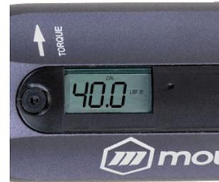
The value displayed when selecting the model is the max range of the tool and displays on whatever units were selected before. If you are calibrating an FGA-8 in cN.m, you need to choose the maximum capacity for that model in cN.m torque unit.
