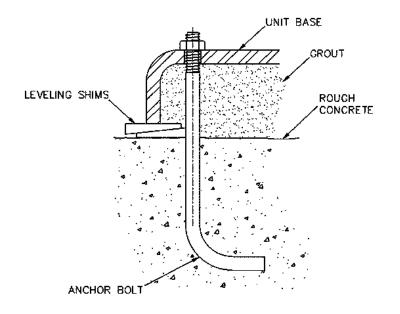
Figure I-1: Typical Anchor Bolt Detail
