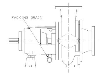
Figure I-6: Packing Drain
