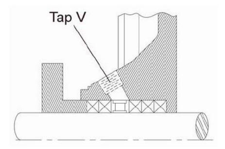
Figure I-5: Packing Flush Connection
