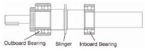
Figure V-1: Typical Shaft Arrangement
