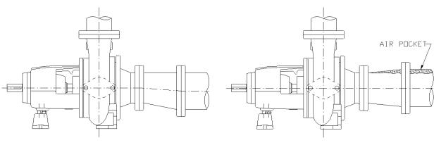
Figure I-3: Recommended Suction Piping
