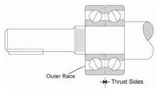
Figure V-3: Duplex Angular Contact Bearings
