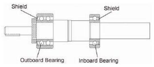
Figure V-2: Shielded Bearing Arrangement
