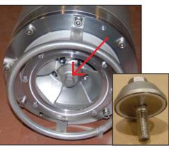
TK150: Remove impeller nut with bolt and o-ring to check cofferdam. Reinstall using Loctite 222 and 68 Nm torque.
