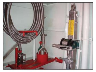
The pump and hoses must always be safely supported and fastened in order to avoid wear or damages due to ship movements. It is especially important that the hoses are not hanging or laying over sharp edges, or that sharp objects are placed upon them. The bending radius for the hoses during storage must not be less then specified.
