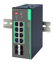
POE-SWR608G is a Web Smart PoE industrial switch, with eight 10M/100M/1000Mbps adaptive RJ45 ports and four 1000Mbps SFP optical fiber module expansion slots. All eight RJ45 ports support PoE/PoE+ power supply. It supports static routing, provides comprehensive security policies, QoS policies, and rich VLAN functions. It has the ring network function and can form a ring network. Switches hold hands to form a ring network topology.
