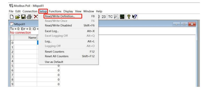
Set the default slave ID(2-in-1 is 44,5-in-1 is 10, 7-in-1 is 20), function code 04, starting address 0, quantity (2-in-1 is 12, 5-in-1 is 6, 7-in-1 is 28);
