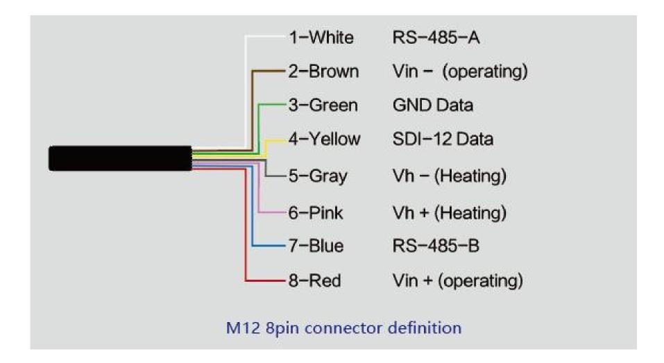
The device adopts an M12 8-pin connector, the different colored pins provide power and data communication (as shown in the above diagram).
