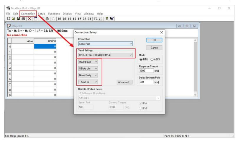
Read the air temperature register 0x0000 to 0x0001, click Setup, and select Read/Write Definition
