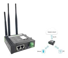
IOT-4GW01 is an industrial 4G LTE router for North American and Australia which supports WAN, LAN, WLAN and 4G interface. User can access to 3G/4G network by WLAN interface or Ethernet interface.
