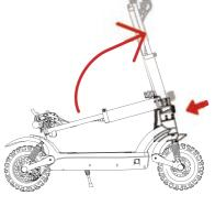
2. Press the folding mechanism and lift the T-bar upright. Push down the kickstand.
