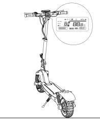
1. Turn the power on, and check the battery level indicator.
