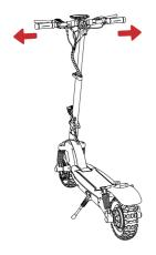
3. Cut the tapes on the handlebar.Lift the handlebars on both sides up and slide in to secure. (Tips: Don't tighten only one side one time, visit www.iscooter.com for additional help with assembly, including a step-by-step video.)
