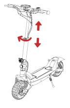
4. Open the adjustable lock, adjust the handlebar to the height you needed, then close the lock.
