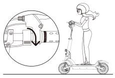
3. When the scooter starts to move forward, put both feet on the deck and press the accelerator. (The accelerator initiates once the speed exceeds 3 mph.)
