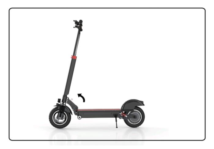
Step 3: Expand the handlebar upward and keep it straight.
