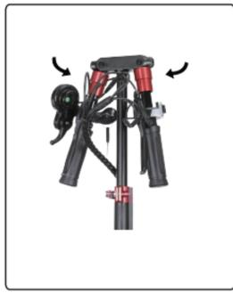
Step 2: Release the quick release clamp on the front tube. Press down the handlebar to the bottom.
