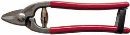
1330 Wire hand shear Forged metal body, cold-protective, coating, suitable for soft wire
