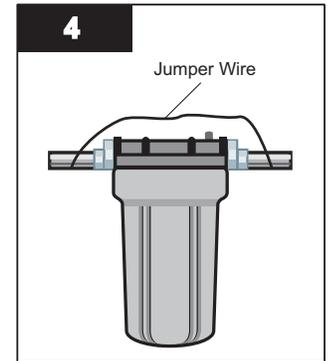
**Note:** If water pipes are used to ground electrical system, appliances, or phone, install a jumper wire.
