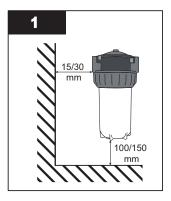
Install the filters at a minimum distance of 15-30 mm from the wall and 100-150 mm from the ground.
