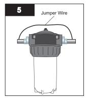
**Note:** If water pipes are used to ground electrical system, appliances, or phone, install a jumper wire.
