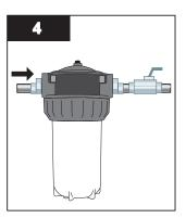
Connect and tighten, making sure filter is in a straight vertical position.
