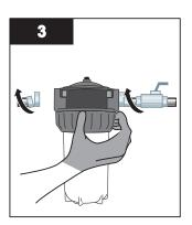
Screw filter to the adapter after covering the threads with Teflon<sup>™</sup> tape and make a tight connection but do not over tighten.
