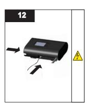
Plug in power cord and sensor cable (if equipped).
