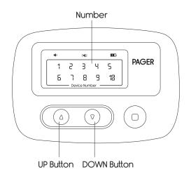
**Step 3:** There are 10 channels on the pager for programming up to 10 individual wireless devices. Select a number for programming by pressing the UP or DOWN arrow on the front of the pager.
