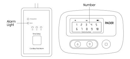
**Step 4:** While the pager is in pairing mode, a red light should flash over the device number (#1-10) that you are attempting to pair the alarm with. While this light is flashing, press the button on the transmitter once to wake it up, then hold for 5 seconds until the alarm light on the transmitter flashes orange. Then release the button on the transmitter.
