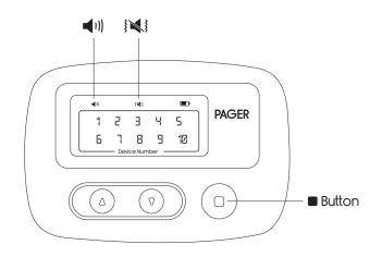
To select another notification mode, press and release the UP Button or DOWN Button on the front of the WPG. The next notification light is will start blinking. Continue to press and release the Up or Down buttons until the desired notification light is selected. Once you've landed on your desired notification light, press and release the Button, you will hear a 1 second beep and/ or feel a 1 second vibration. This means the current notification mode is recorded to the WPG.
