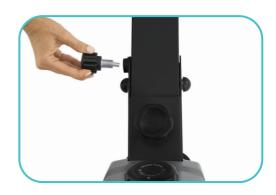
15. Fit a Large Flat Washer over the end of each Long Hex Bolt, and fit them through the bolt loop on the Foot Pedals and into the screw holes on the sides of the Mechanism Housing. Tighten with the wrench, making sure the textured side of the pedals are facing the Slide Rail, and the heel rest is on the bottom.
