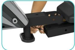
11. Slide the rail upwards so that the screw holes on the top and sides of the rail are aligned with the bracket holes from the housing piece. Place a Flat Washer over the end of each screw hole on the sides of the rail, and fit the Medium Hex Bolt through to hold the rail in place. Secure the bolt in place with the Hex Nut and tighten.
