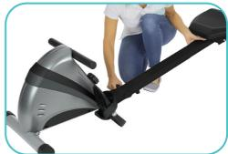
3. Lift the Slide Rail up to a vertical position, where the hole in the Angle Plate on the bottom of the Slide Rail aligns with the Positioning Knob screw hole. The Positioning knob will pop back into place locking it in the upright position. You can retighten the positioning knob with a clockwise turn for a better hold.
