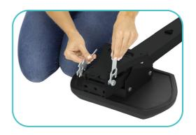
8. Attach the Stand Cover to the outside of the Rail Stand, and secure in place by fit the Connecting Knob into the hole at the end of the Slide Rail.
