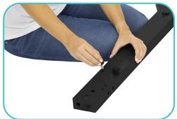
4. Fit the Slide Seat over the end of the Slide Rail where the plate and stoppers were just removed. The seat should be fitted on wide side first, so that the seat pad is on the side of the rail opposite the removed cushions and angle plate.
