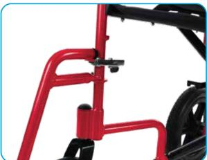
To remove the foot rests, pull the wide end of the silver clasp in towards the middle of the chair. You will feel the clasp release its grip on the frame, and the foot rest will swing out where it can be lifted off the two metal placement pins.
