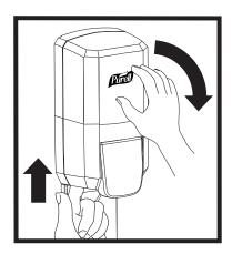
**1.** Open dispenser by depressing release button on bottom and pull down on fron cover.
