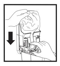
**2.** Remove refill from shipper and insert into dispenser with nozzle in front.
