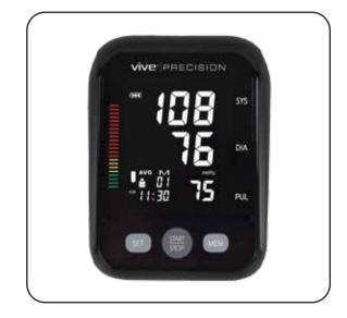
Repeat Step 1 to set MONTH DAY, HOUR, MINUTE, TIME UNIT and PRESSURE UNIT. Note: A normal blood pressure range is 120 / 80 mmHg.
