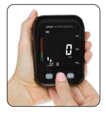
When a pulse is detected, a heart symbol will flash on screen.
