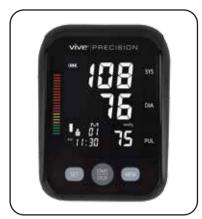
Press and release the MEM button again to see the most recent measurement. Press and release the MEM button again to scroll through older measurements.
