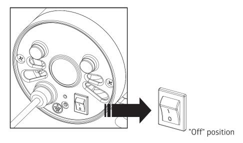
2. Switch the power switch to "I" position (on), the unit start running.
