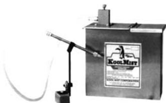
Model KM100N with 1 outlet shown with magnetic positioner No. KM 205
