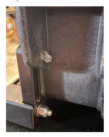
17. Install a 35mm bolt, nut, large washer, and small washer as shown below. Note the large washer is located on the inside and the small washer is located on the outside. Ensure the gaps are even in all 4 locations as per step #12, tighten fully. Note that the large inner washer may start to embed itself into the box flange – try to keep this to a minimum.
