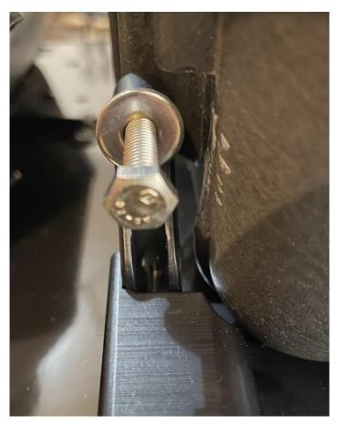
20. While holding the washer flush against the link, push the link towards the box until the washer contacts the box. The washer is serving as a spacer for locating the link.
