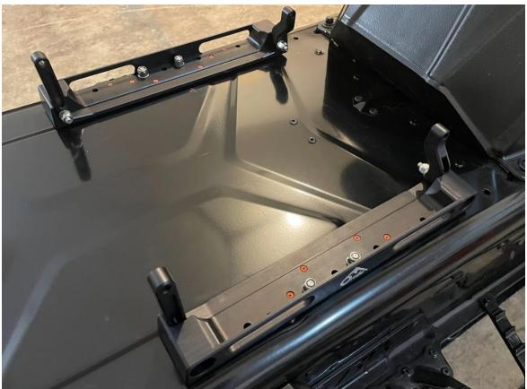
10. Place the box down on the mounts, ensure that all the links line up with their respective box flanges as shown.
