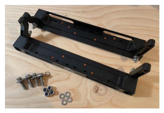
9. Install the mounts onto the tunnel, but only tighten the nuts until they are flush with the top of the bolts. The large washer goes under the tunnel, and the small washer and nut go on top of the mount. Note the bent links connect to the back of the box, so consider which box orientation you want when mounting for ease of access to the box contents.
