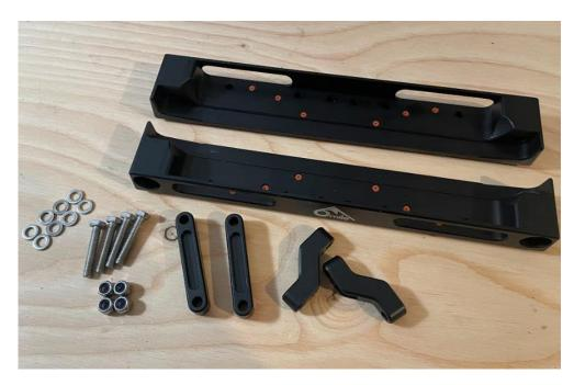
7. Install the links as shown, but only softly snug the bolts so that the links still move with a small amount of force.
