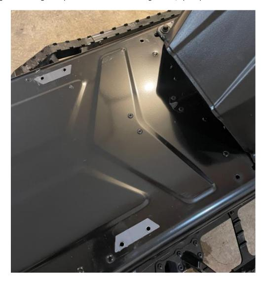
5. Place the mount bases over the holes and observe if any high spots on the tunnel are causing the orange pads to not all sit flush as shown below. Notice that there is an air gap under all the pads indicated by yellow arrows because the pad with the red arrow is high centered.
