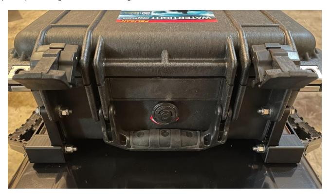
19. Ensure that the gaps from step #12 are still even, then place a 35mm bolt with a large washer into one of the bent links. The bolt will stop when it contacts the flange.
