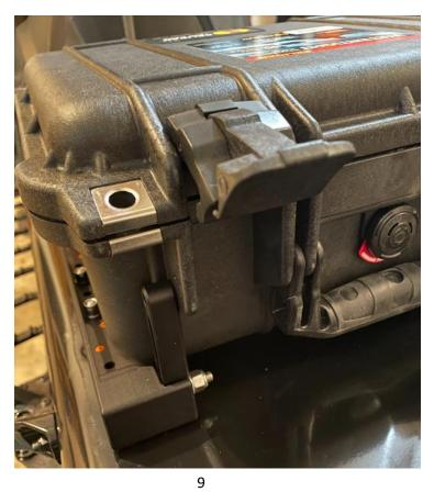
12. Observe the gaps between the front of the box and the mount, and between the back of the box and the mount in the locations shown and adjust the box position until the gaps are even on both mount bases (4 locations total).
