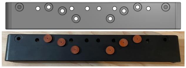
3. Place the mount bases on the tunnel and position them over the tunnel mounting holes using one of the hole pairings shown below to determine which location works best for your application.
