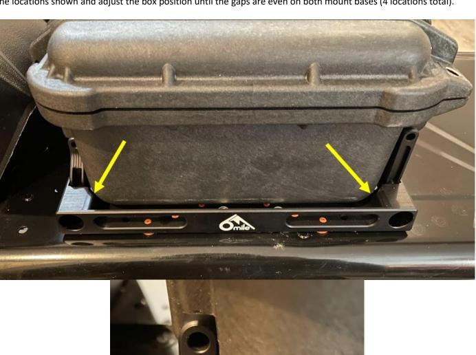
13. While ensuring the box doesn't move and the gaps are even in all 4 locations as per step #12, press one of the straight links towards the box until it comes into contact with the box.
