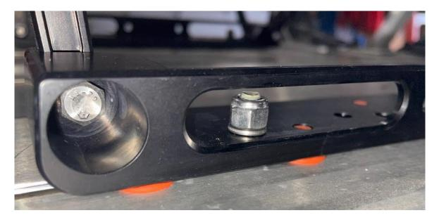
8. Place the box down on the mounts, ensure that all the links line up with their respective box flanges as shown.
