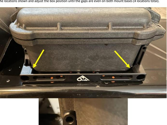
11. While ensuring the box doesn't move and the gaps are even in all 4 locations as per step #10, press one of the straight links towards the box until it comes into contact with the box.
