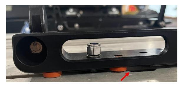
7. Ensure the mounts are lined up directly across from each other on the tunnel. Tighten the mounts down fully. Alternate back and forth between the two bolts on each mount base until both are tight, paying close attention to the rubber bumpers. As you tighten, they will start to squish, you will have sufficiently tightened far before the nut feels tight, as you're only trying to achieve a slight compression on the pads, you do not want to fully squish them flat.
