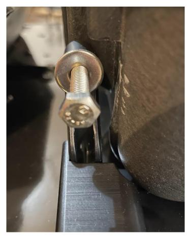
18. While holding the washer flush against the link, push the link towards the box until the washer contacts the box. The washer is serving as a spacer for locating the link.
