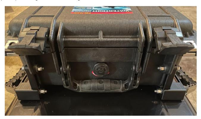
17. Ensure that the gaps from step #10 are still even, then place a 35mm bolt with a large washer into one of the bent links. The bolt will stop when it contacts the flange.
