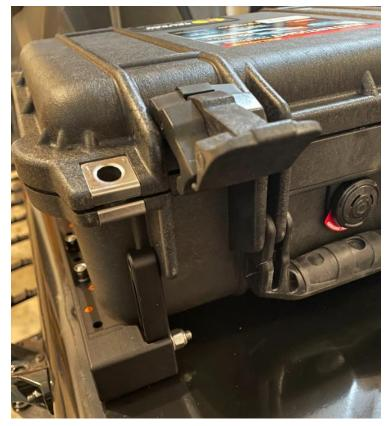
10. Observe the gaps between the front of the box and the mount, and between the back of the box and the mount in the locations shown and adjust the box position until the gaps are even on both mount bases (4 locations total).
