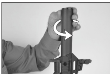
3) Take out the Muzzle Brake by turning counterclockwise
