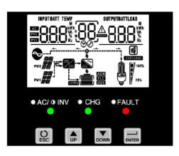
AC / INV - green solid LED = Mains is powering AC output (AC throughput mode)
