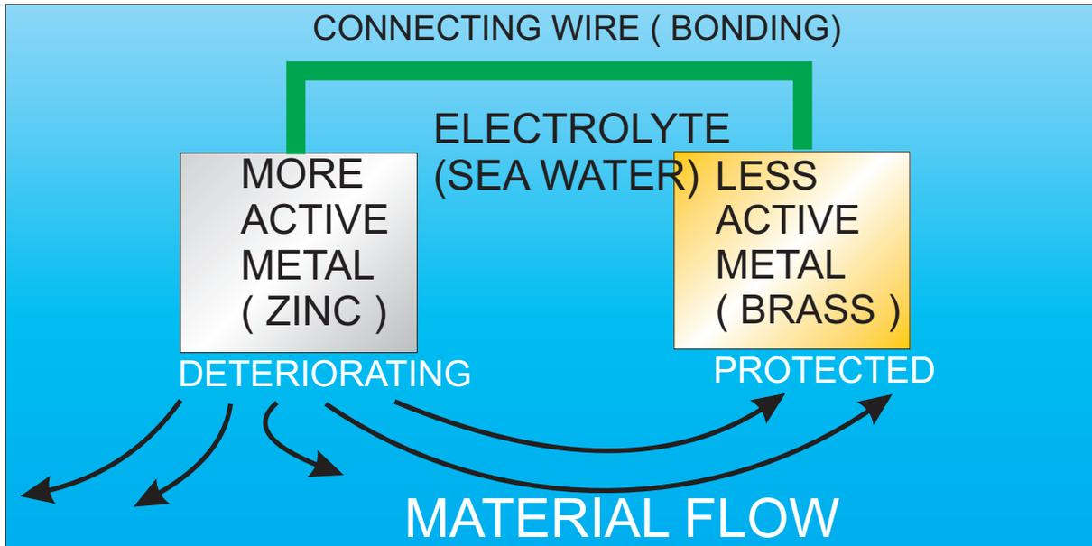
If both the above metals were important to us, we could attach a third metal say magnesium to the bonding wire this would mean that all the magnesium would deteriorate before the zinc, then the brass.
