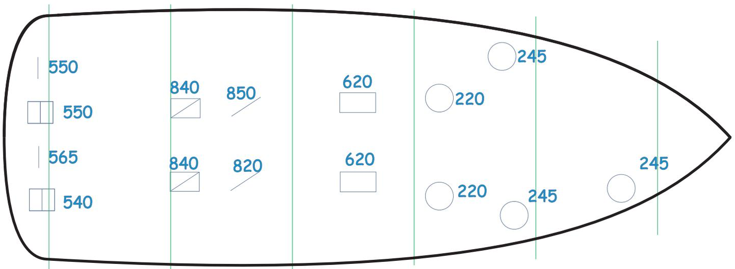
Remember the engine has its own body of water and protection. your half cell is not in its body of water so engine readings do not reflect conditions inside the engine, Check the engine zincs visually. All the bronze fittings are in the 'freely eroding' range. After bonding, the readings at each piece should be the same.
