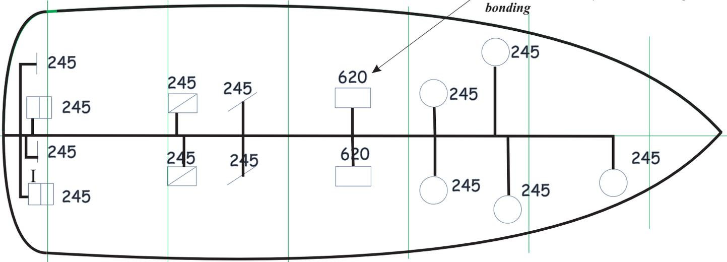
Install a sacrificial anode (normally zinc) to the bonded boat.
