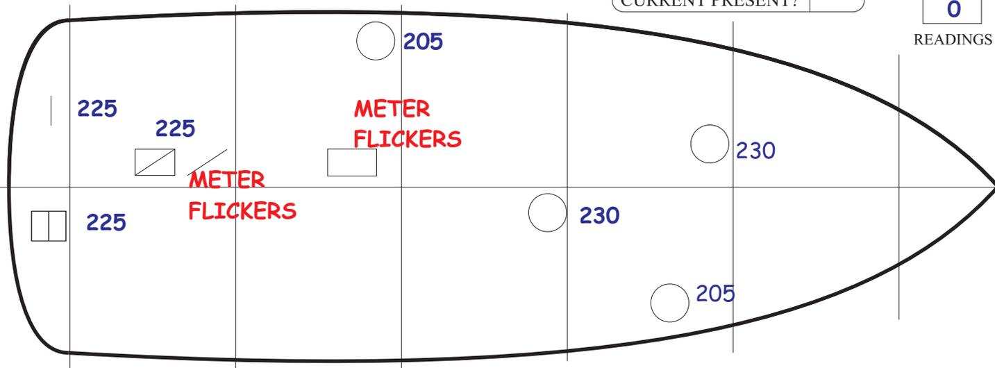
Results **NO BONDING / HOT WIRE ON A.C. SHORE CORD CONNECTED TO ENGINE AND PROPSHAFTS**
