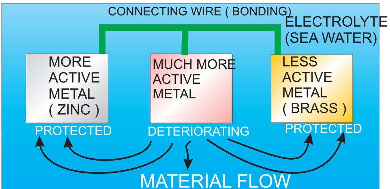
If we know that the metal that is most active electrically will deteriorate while protecting the metal that is less active it is important that the most active metal is not an important part of the boat.
