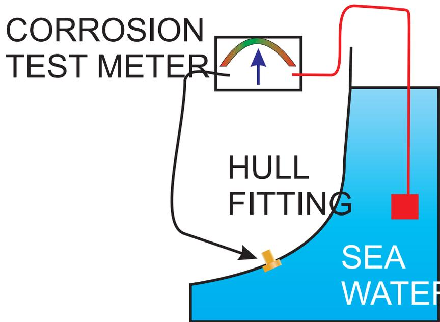
The 'Corrosion Test Meter' consists of a highly accurate millivolt meter, a probe and a silver/silver chloride half cell. Other less expensive half cells could be used but they do not have the stability or the reliable readings of silver/silver chloride.
