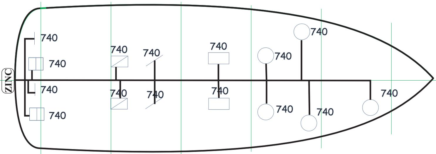
If the zinc is large enough, the voltage will be in the green or higher (500 to 900 millivolts on bronze) and will protect the boat metal until the voltage drops to within 200 millivolts of its 'freely eroding' voltage
